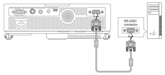
Serial cable (D-Sub 9-pin, straight) (commercially available)
